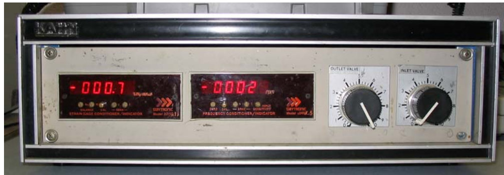
Figure 2.1.2. Kahn Manual Remote Dynamometer Control System (Photo: Matthew Zimmer)
